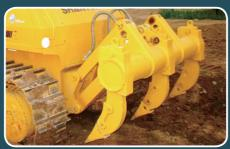
Three-shank aggressive parallelogram ripper lets you do more be used for self rescue, productive ripper work. The parallel linkage design provides better penetration and maneuverability in tight working areas.
