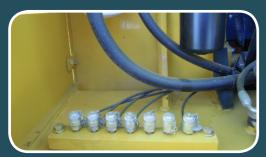
Grouped pressure taps for quick testing and troubleshooting of the hydraulic system.
