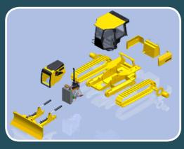
\*Modular design allows the components to be easily accessed, removed and installed without spilling oil. This can further help reduce downtime and enhance serviceability.
