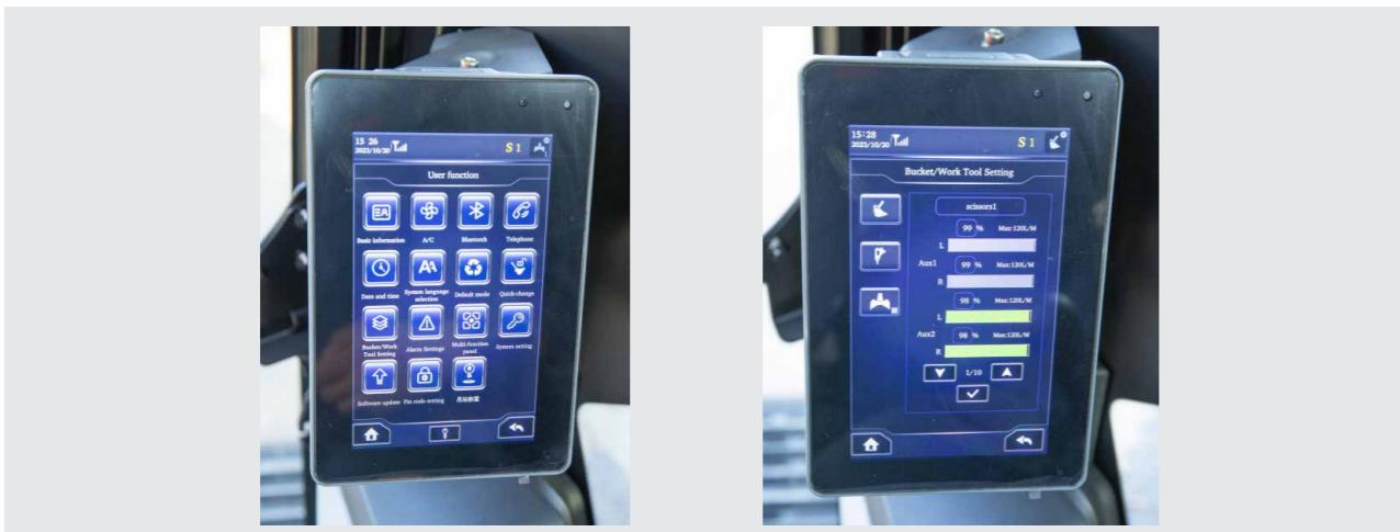
A monitor with a high-resolution display shows all important data at a glance. The menu navigation is extremely user-friendly and enables the driver to manage machine functions safely and comfortably. The camera image can also be shown on the display if required. The next inspection due and basic data such as torque and oil and cooling water temperatures are also displayed.
